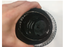
Hold Handle Firmly and Pull Up
