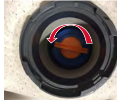
Turn Filters Counter-clockwise to Remove
