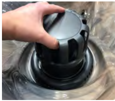
Pull Up to Remove Floater Assembly
