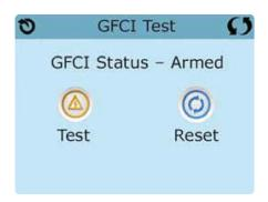
The Ground Fault Circuit Interrupter (GFCI) or Residual Current Detector (RCD) is an important safety device and is required equipment on a hot tub installation.
