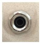
**7. 3-WAY DIVERTER JET** (if equipped, GetAway Hot Tubs) This large jet can be turned 180° to 3 different points and diverts the flow of water from one group of jets to another. With the pump turned off, twist the face of this jet 1/4 turn at a time clockwise or counterclockwise to adjust.
