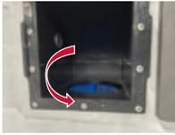
*Turn Filter Counter-clockwise to Remove*
