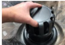
*Pull Up to Remove Floater Assembly*
