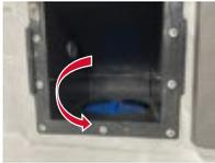
*Turn Filter Counter-clockwise to Remove*
