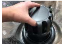
Pull Up to Remove Floater Assembly
