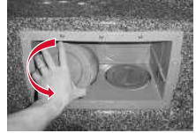
Turn Filter Counter-clockwise to Remove
