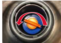
Turn Filters Counter-clockwise to Remove
