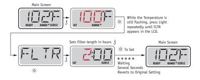
If Filter Cycle 2 is enabled, Filter 12 will appear in the LCD. If Filter is disabled, Filter 1 will appear.
