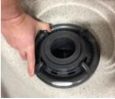
Twist Lock Ring Counter-clockwise to Remove Floater
