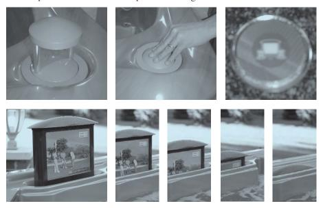
The TV and pop up speakers can be raised and lowered by pressing the one touch up and down FST auxillary button. Be sure the TV and speakers are down before placing the cover on the spa. Resulting damage is not covered under warranty if the cover is installed while the TV and speakers are still in the upright position.
