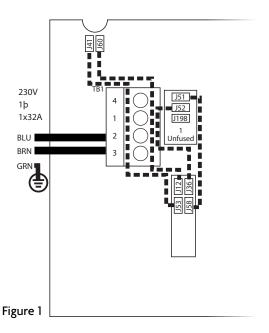
\*Wiring must be sized to swim spa specification. Swim spa rated maximum ampacity cannot exceed the service maximum ampacity. This does not represent an option to the Installer. See Model Specifications page for electrical requirements by spa model.
