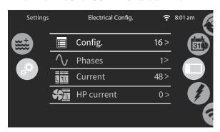
To make alterations to the electrical configuration of your swim spa naviagte to the Electrical Config. section of the Setting Menu. However, before making any changes either contact a Master Spas Customer Technician or a Licensed Electrician. In order to make changes you will need a passcode which is **5555**.
