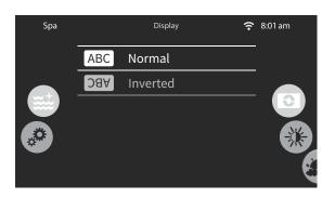
**Inverted** screen display orientation allows you to flip the display 180 degrees.
