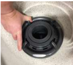
Twist Lock Ring Counter-clockwise to Remove Floater
