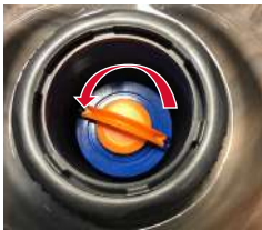
Turn Filters Counter-clockwise to Remove
