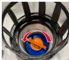
Turn Filters Counter-clockwise to Remove
