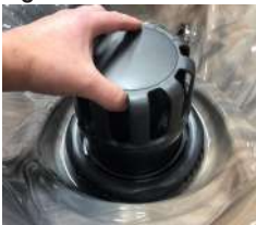
Pull Up to Remove Floater Assembly
