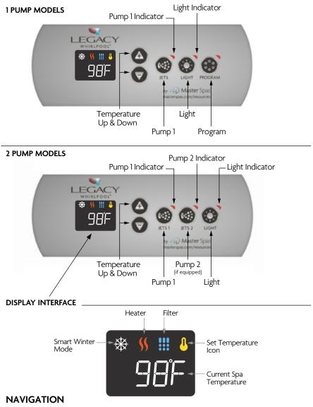
Navigating the entire menu structure is done with 2 or 3 buttons on the control panel. To start or stop a feature, press the associated button. Red indicators
