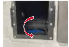
Turn Filter Counter-clockwise to Remove
