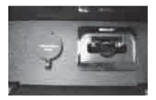
We have installed an F-81 television coaxial cable connector located under the front panel for your convenience. This can be utilized if you wish to add a cable connection or satellite connection to your STS.
