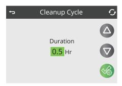
**NOTE:** Cleanup cycles do not apply to systems set for 24hr circulation pump mode as the circulation pump performs as the heat and filter pump to provide constant filtration.
