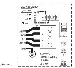
\*Wiring must be sized to swim spa specification. Swim spa rated maximum ampacity cannot exceed the service maximum ampacity. This does not represent an option to the Installer. See
