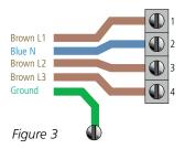
\*Must be sized to spa specification. Spa rated maximum ampacity cannot exceed the service maximum ampacity. This does not represent an option to the Installer.
