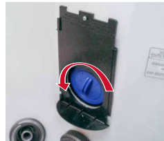
Turn Filters Counter-clockwise to Remove
